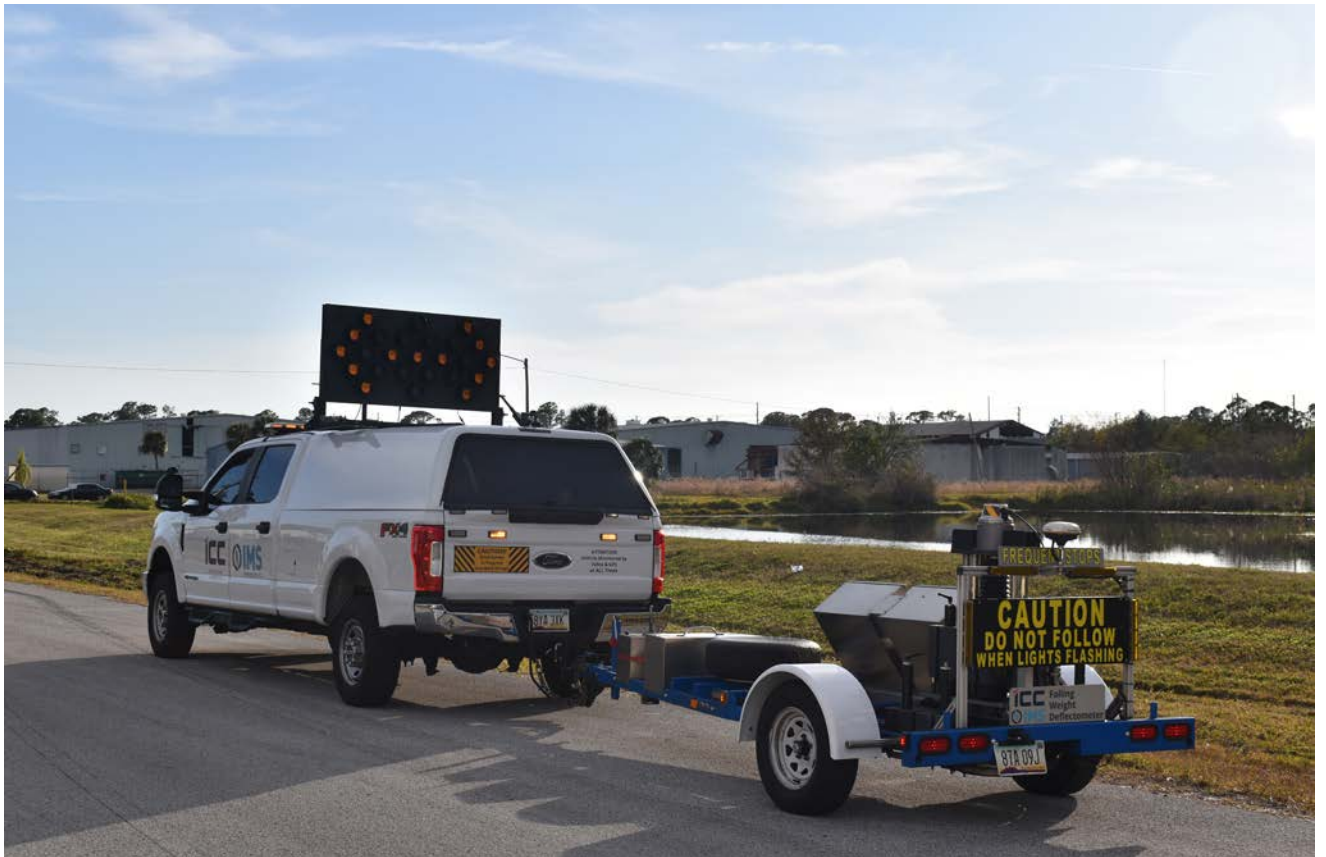
Assessing pavement load-bearing capacity using a Falling Weight Deflectometer (FWD)
