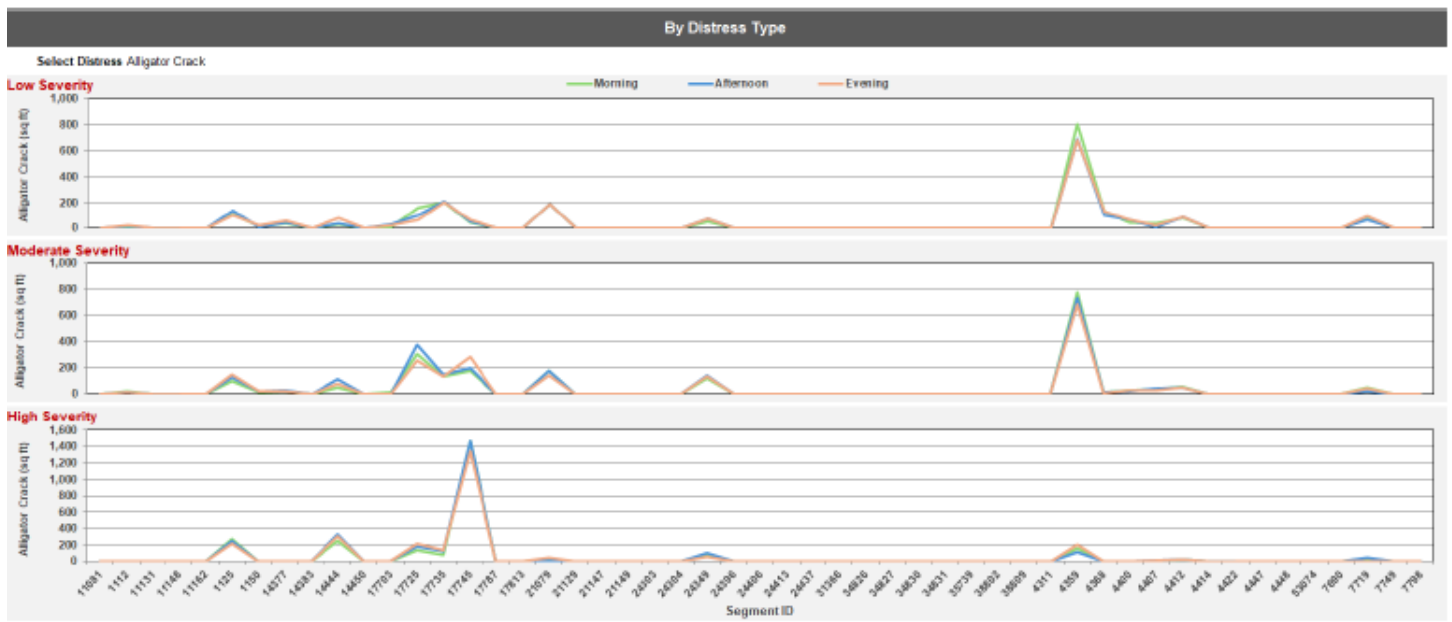
Figure 4: Alligator cracking comparison by segment
