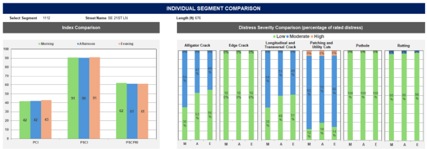
Figure 5: Summary condition index and detailed distress comparison for a single segment
